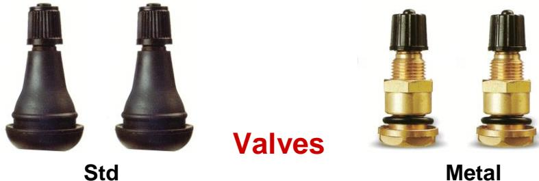
Standard rubber valves designed for passenger cars have a maximum pressure of 450 kPa with hot tyres. Vans, mobile homes and caravans with C-tyres must have a screw (metal) valve or a special high-pressure valve, if tyre pressure exceeds 450 kPa with a hot tyre. If ordinary car valves are used, there is a high risk of them starting to leak air at high pressures. It is a good rule never to use car valves on C-tyres.
